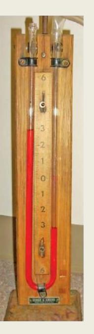
A manometer is used to measure the pressure of a gas in a tank. The fluid used has a specific gravity of 0.85, and the manometer column height is 55 cm. If the local atmospheric pressure is 96 kPa, determine the absolute pressure within the tank.
