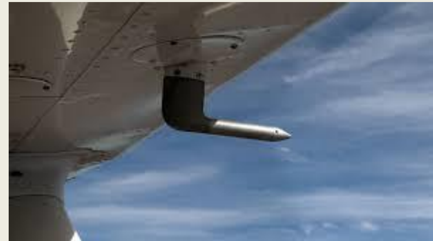
Pitot tube installed on a plane
