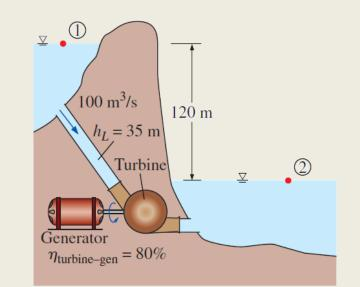
$$\frac{P_1}{\rho g} + \alpha_1 \frac{V_1^2}{2g} + z_1 + h_{\text{pump}, u} = \frac{P_2}{\rho g} + \alpha_2 \frac{V_2^2}{2g} + z_2^2 + h_{\text{turbine}, e} + h_L$$
