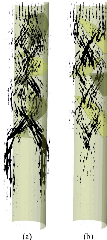
Fig. 3. Time averaged velocity fields (a) 180° Kenics static mixer (b) 45° LPD static mixer.
